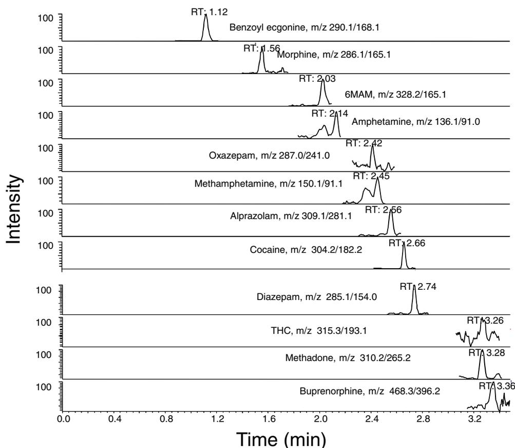
**Figure 2.** Chromatograms from an extracted filter fortified with all analytes at the LLOQ levels (see table 3). The chromatograms represent results from the quantifier transitions (product ion 1 of table 2).
