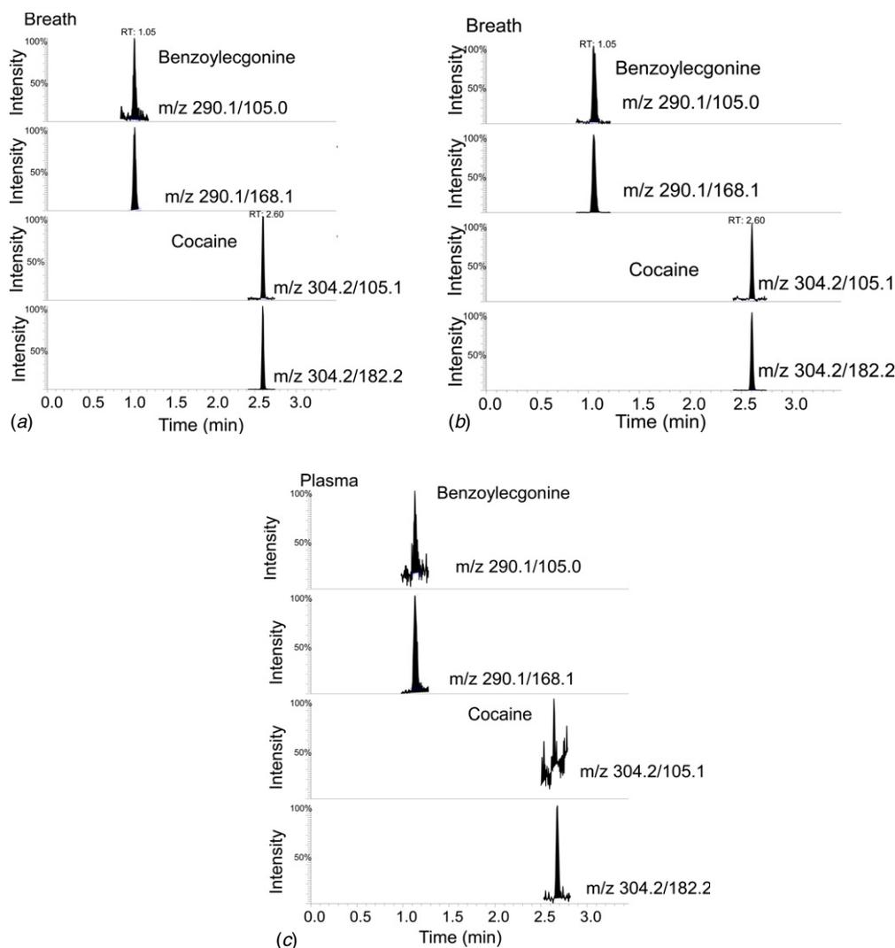
**Figure 4.** Chromatograms obtained from the analysis of benzoylcegonine and cocaine in exhaled breath ((a) case 2; (b) case 14 of table 7) and plasma ((c) case 14) using electrospray LC-MS/MS and monitoring of two product ions from each of the protonated molecular species. Note that the chromatograms shown for benzoylcegonine in 4(a) and both analytes in 4(c) represent concentrations below LLOQ.
