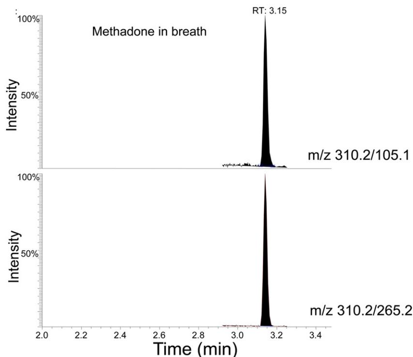
**Figure 3.** Chromatograms obtained from the analysis of methadone (case 8 of table 4) in exhaled breath using electrospray LC-MS/MS and monitoring of two product ions from the protonated molecular specie.
