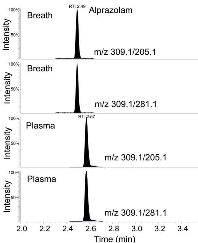
**Figure 5.** Chromatograms obtained from the analysis of alprazolam in exhaled breath and plasma (case 31 of table 10) using electrospray LC-MS/MS and monitoring of two product ions from the protonated molecular specie. The difference in retention time between breath and plasma was due to the fact that two different set of instruments were used.
